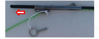
3. Push the wand tube assembly into the groove on the bow mechanism and push the fast pin into the holes to connect both components together.
