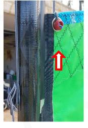
3. When the sail is fully raised, insert the knot into the halyard lock on the front side of the mast.
