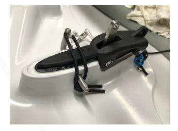
4. Once in deep water, open the clamp and push the centreboard fully down and insert the retaining pin through the hole in the foil case and centreboard. Pull the shock cord attached to the retaining pin over the rudder and over the other end of the retaining pin.
