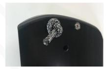
5. To lock the rudder into place, pull the retaining toggle pin over the top of the rudder and onto the opposite side of the rudder box. Insert it through the rudder box and rudder hole. Make sure the toggle pin nose drops to be engaged properly.
