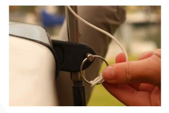
4. Run the wand rope around the boat, threading the wand cord through the fairleads and pulleys as shown below.
