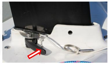
3. When leaving the shore, use the foil clamp to hold the centreboard at the appropriate height to safely leave the shore. Once in deep water, open the clamp and push the centreboard fully down and insert the retaining pin through the hole in the foil case and centreboard. Pull the shock cord attached to the retaining pin over the top of the centreboard and over the other end of the retaining pin.
