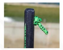
The wand is now ready for use, pull the cord to raise or lower the wand. This changes the ride height whilst sailing.
