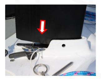
2. Attach the horizontal main foil under the boat whilst on the trolley by aligning the pins, press the push button in and slide the foil it up into place.
