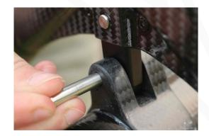
2. To attach the stays onto the spreader;
