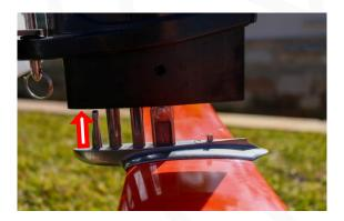
3. Clamp the rudder in place using the toggle clamp.
