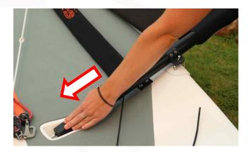
3. The outer pin will sit inside the hole on the moulding attached to the rear bar. Push the retaining pin in place.
