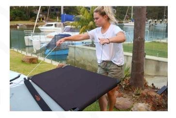
**To remove wings:** Undo the retaining fast pin, pull the rear wing bar out and away from the hull. When clear of the 2 attachment pins, lift the rear wing bar upwards. Then slide the front of the wing outwards and away from the hull – the wing should come away easily.
