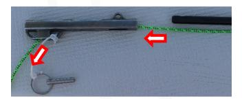
2. Insert the wand inside the wand tube assembly, ensuring the rope is sitting in the groove at the back of the wand.
